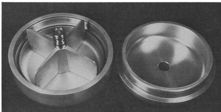
Fig. 3. Components of the B-XV zonal rotor. The rotor chamber consists of two similar halves which thread together. The static seal is not shown. (Scale: \frac{1}{4} cm = \sim 1 cm)
