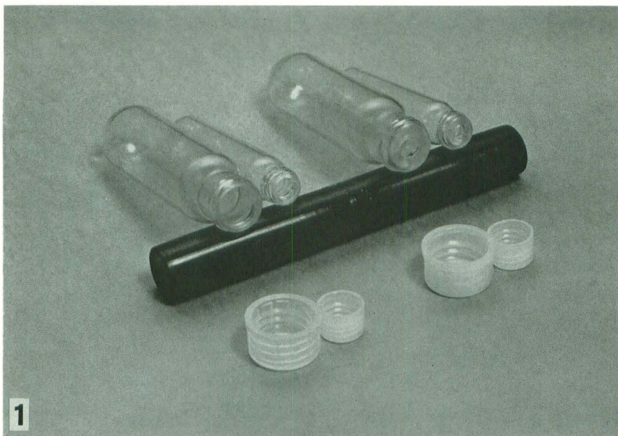
FIGURE 1.—Plastic ultracentrifuge tubes. Type A (small opening for virus isolation) shown on right , type B (large opening) shown on left .
