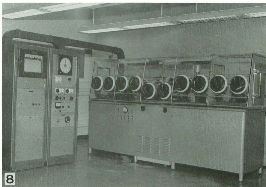
FIGURE 8.—Containment system for zonal centrifuge (installed at plant of Charles Pfizer and Co., Maywood, N.J.).
