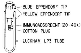
FIG. 1. Diagram of microimmunoabsorbent column. A section of the large end of a blue Eppendorf tip serves as an adaptor holding the yellow tip column. A firm cotton plug holds the immunoabsorbent in place. This arrangement can be centrifuged to dry the immunoabsorbent and, after rehydration with one column volume of a dissociating elution buffer, to collect the eluate. Almost all of the bound protein can be eluted in one column volume (20–40  $\mu$ l).
